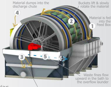
Water & granular solids passing through the bucket sieve mats settle in the bath
