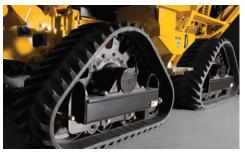
QUAD TRACK ADVANTAGE. The optional quad track system offers improved floatation, reduced surface damage, increased tractive effort and greater stability.
