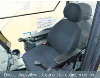
Double slides allow adjustment for optimum comfort
