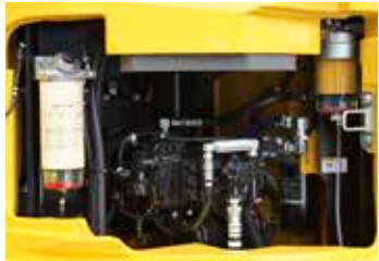
Fuel filter with built-in water-separator
