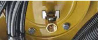
Fuel tank drain valve.
