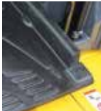
Detachable two-piece floor mat has handles for easy removal. The mat's raised edges trap dirt and grit for easy cleaning.
