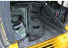
Detachable two-piece floor mat has handles for easy removal. The mat's raised edges trap dirt and grit for easy cleaning.
