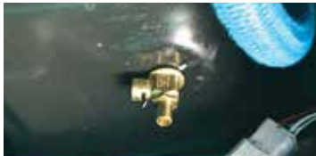
Engine oil quick-drain valve can be turned without, special tools.
