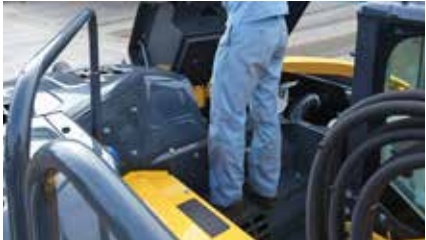
Engine maintenance A special lower access step, near the engine, simplifies maintenance.
