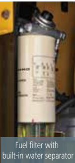
Pre-fuel filter with built-in water separator
