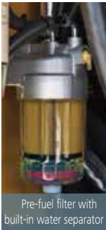
Fuel filter with built-in water separator
