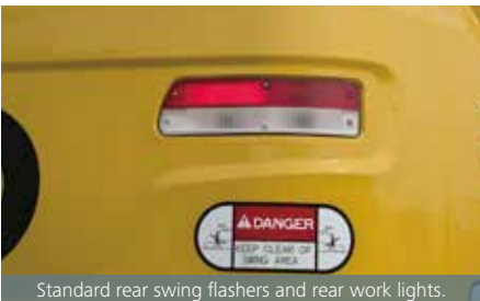
Standard rear swing flashers and rear work lights.
