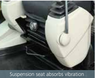
Suspension seat absorbs vibration
