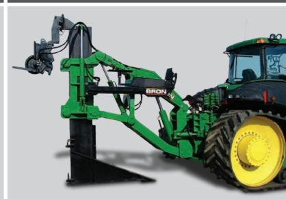
The BRON Add-on Double-Link Plow gets you in the ground as the most economical method of providing accurate tile installation to customers. Available for all sizes of dozers and agricultural tractors, the BRON Add-on Plow has five models for 90-350 HP applications. The quick-attach system makes it easy to disconnect the plow when not in use.
